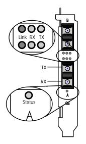
Figure 4. Location of the LEDs (dual link)
